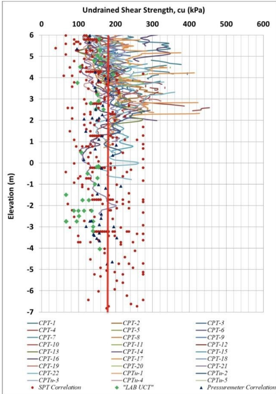
Figure 9-15. Change of Undrained Shear Strength Values with Elevations
